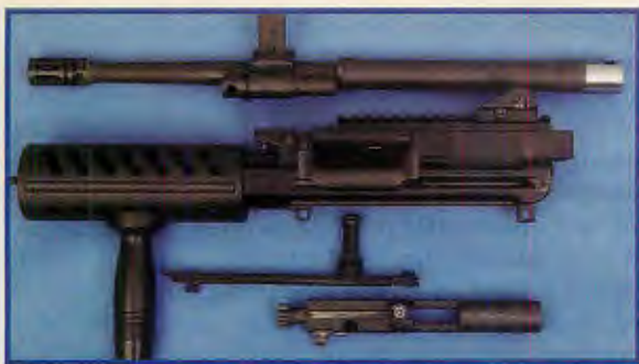
The Shrike upper mates to MilSpec M16/M4 lowers; note quick-change barrel, modified bolt carrier, retracting handle and belt port.
